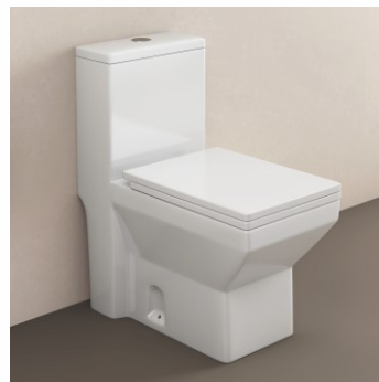
ONE PIECE CLOSET Cat. No. 142 700x360x760mm PP / UF Seat Cover S-Trap Dist. 250mm
