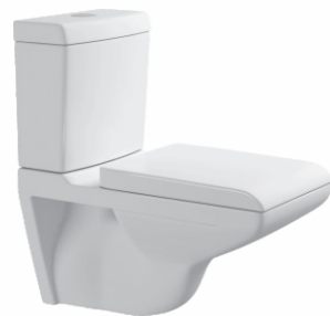
TWO PIECE WALL HUNG CLOSET Cat. No. 10012 _ 660x360x740mm S-Trap Dist. 250/300mm PP Seat Cover
